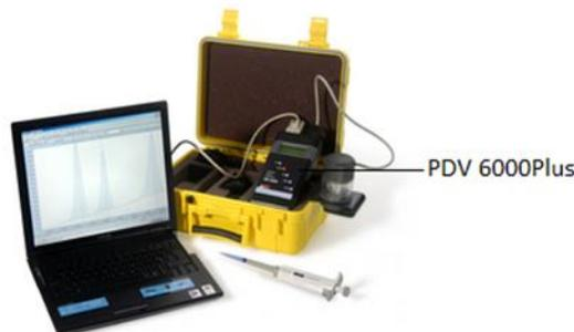
Figure 1 PDV6000Plus and Laptop computer with VAS software
